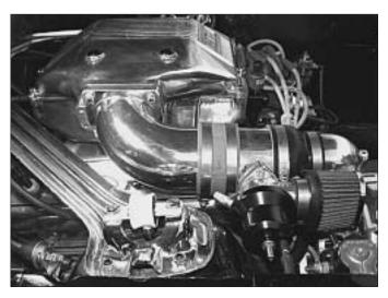
Fig 9-c / Passenger side discharge duct. (1969 351 Mustang)
