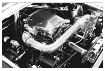
Fig 9-b / Driver side discharge duct. ('64-'68 Mustang)
