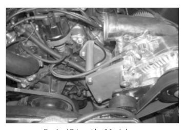
Fig. 6-e / Driver side oil feed shown, passenger's side similar. ('64-'68 Mustang)
