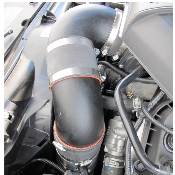
Fig. 7C-7: Cast Elbows, Final Position
