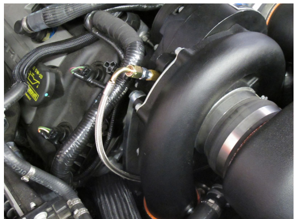
Fig. 13C: 90° Oil Feed Hose Installed
