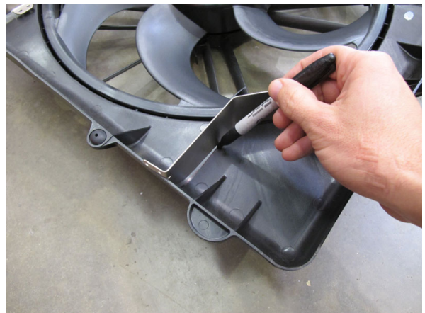
Fig. 3AD: Marking Air Dam Cut Lines
