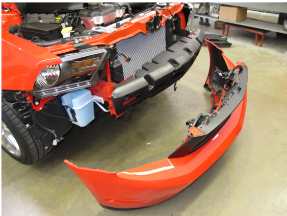
Fig. 1J: Front Fascia Removal
