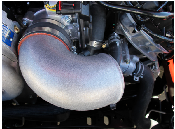
Fig. 7C-6: \text{\O}3.5 " x 120^\circ Cast Aluminum Elbow
