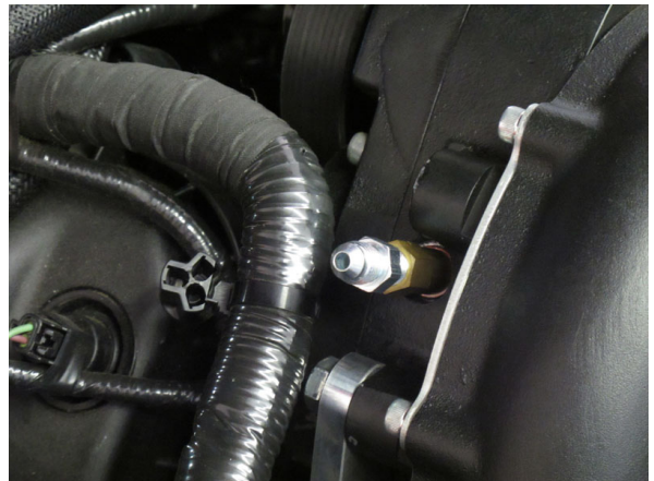
Fig. 13B: -4AN Oil Feed Fitting Installed
