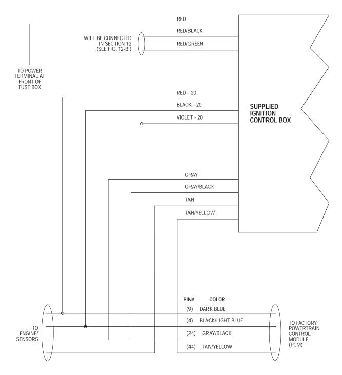
Fig. 11-c / Timing Controller Wiring Schematic
