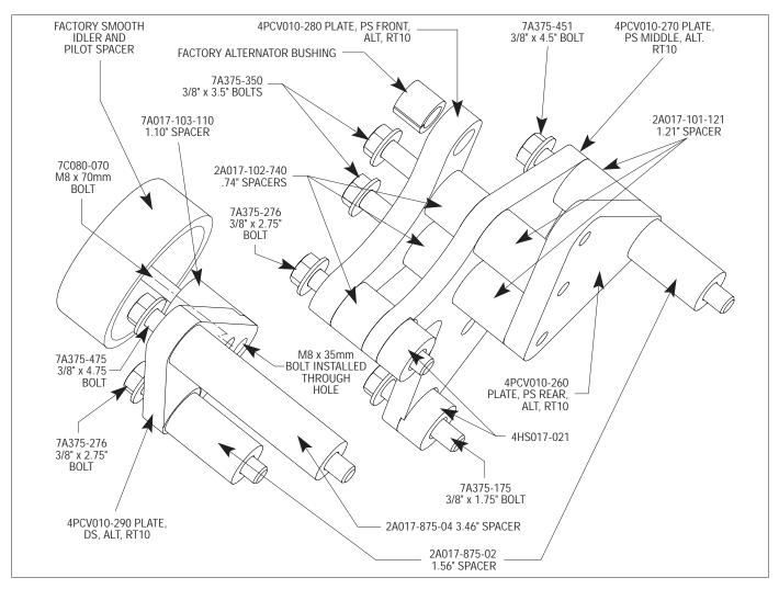
Fig. 7-a | Alternator and spring tensioner not shown
