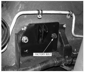
Fig. 5-a / Passenger's side shock tower brace
