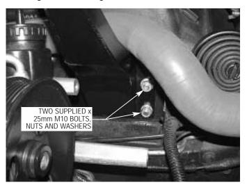
Fig. 5-b / Driver's side shock tower brace
