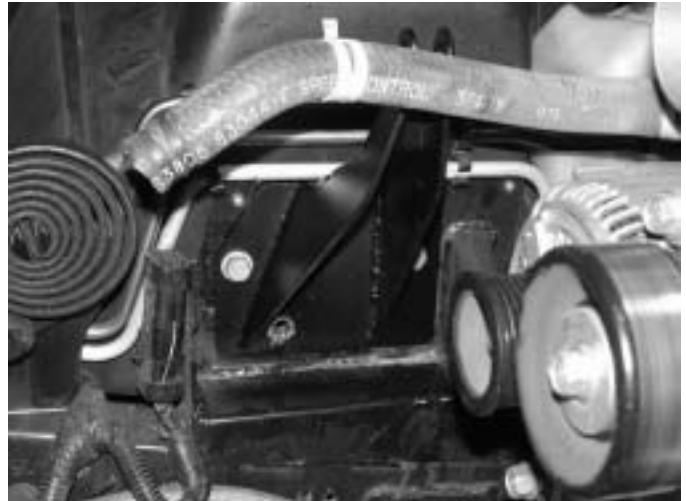
Fig. 5-a / Passenger's side shock tower brace
