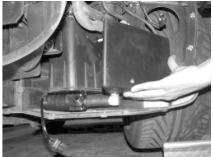
Fig. 9-d-1 (1996-1999 Vehicles) *Installed with 1" NPT Blind Hole Pointing Down
