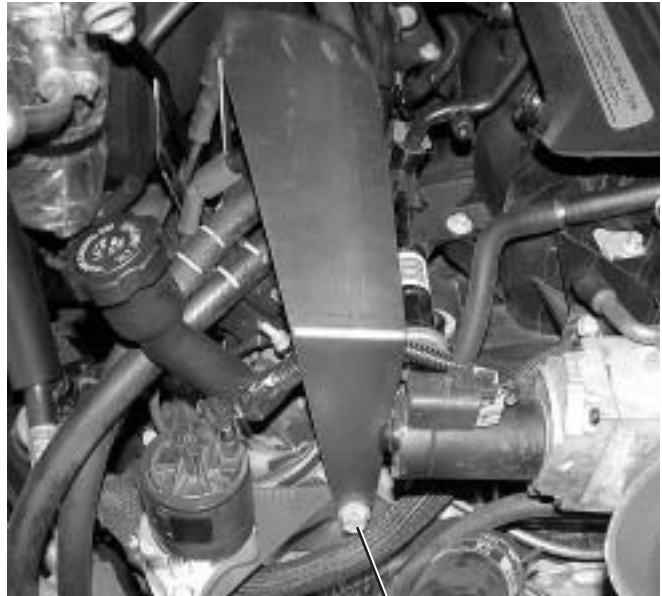
On the H2 Hummer, use the supplied 10mm x 1.5 screw, washer and .975" spacer in place of EGR equipment
