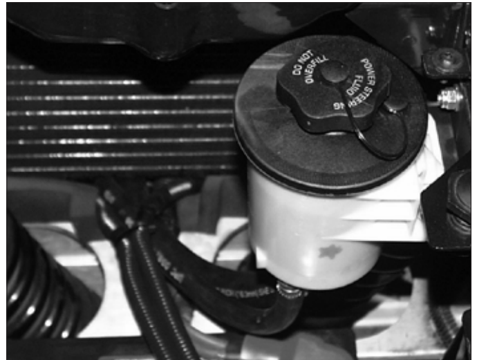
Fig. 5-2 New power steering reservoir, mounted on frame rail. Showing hoses going through the frame.
