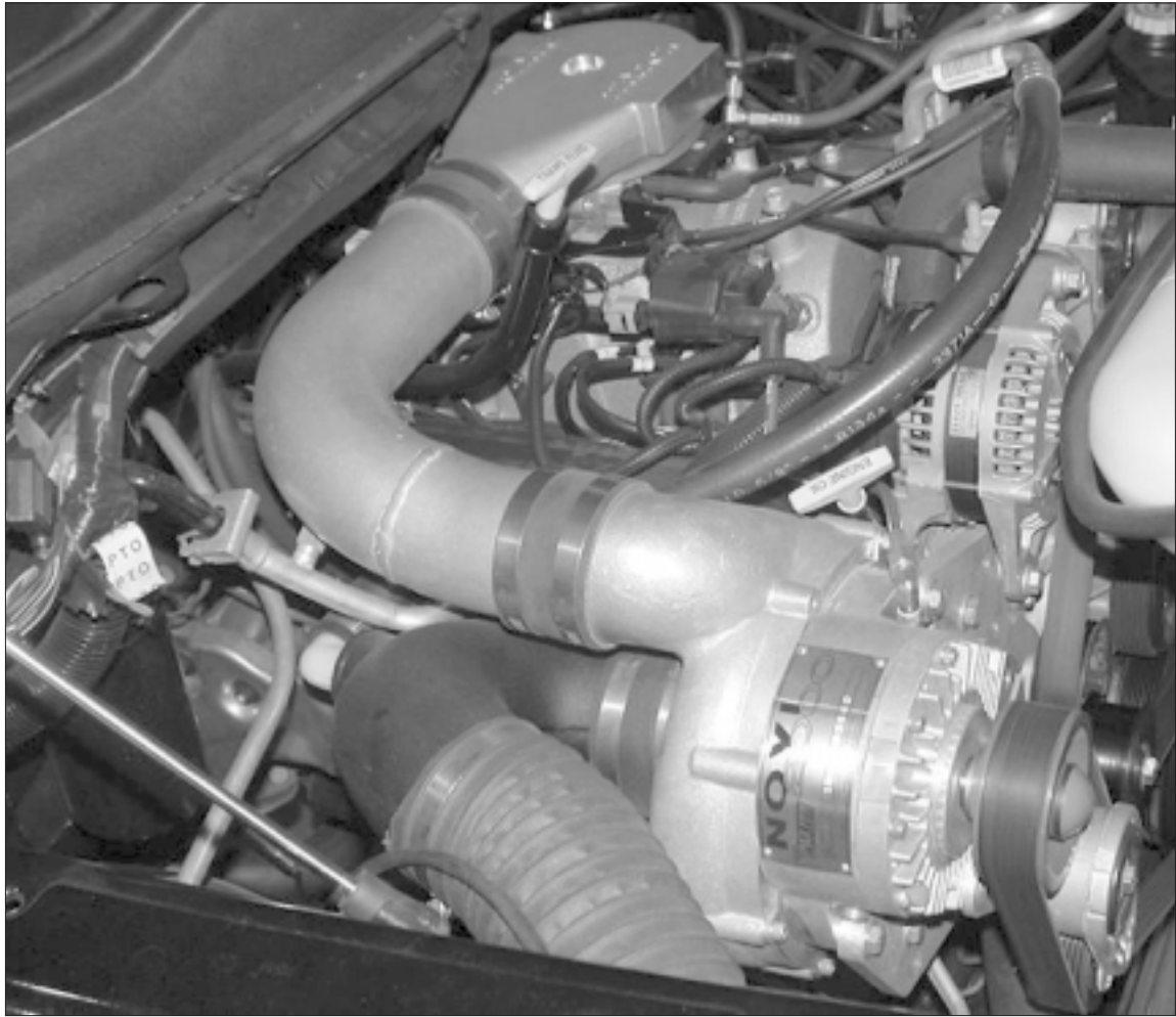
Fig. 8-b / Congratulations - here is your finished supercharged engine.
